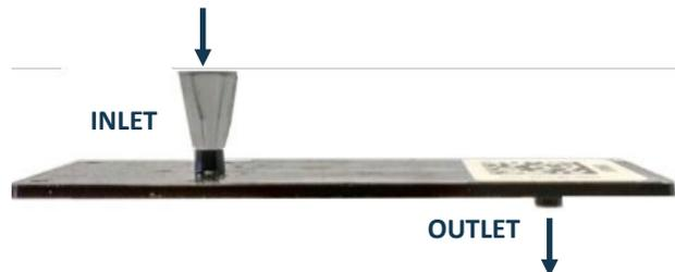
Fig. 2c | ZellSafe™ chip with pipette adapter
