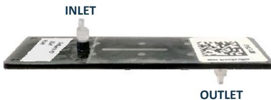
Fig. 2 | ZellSafe™ chip with sealing plugs blocking the inlet and outlet
