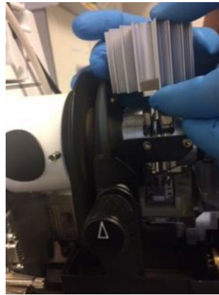
Fig. 5b | Removal of heat sink (Step A7)
