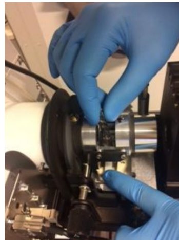
Fig. 6b | Removal of HBO lamp (Step A8)
