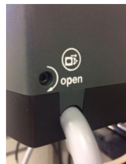
Fig. 3 | Case Screw Location (Step A4)
